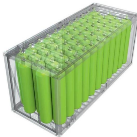
Figure 3. Typical hydrogen storage arrangement
